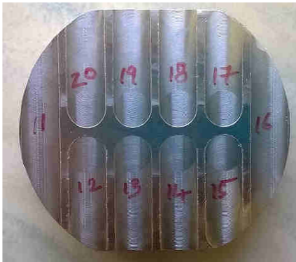
Fig.3: End Mill Slots with 10mm width on Nimonic 75
